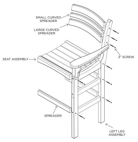
**STEP 2.** Use (8) 3" screws to attach the Right Leg Assembly to the Seat Assembly and spreaders.
