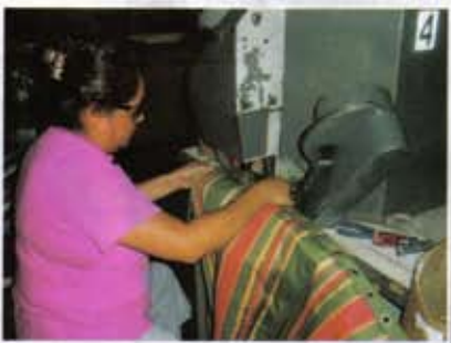
Erika Jimenez applies grommets to edges for hanging a quilted fabric.
